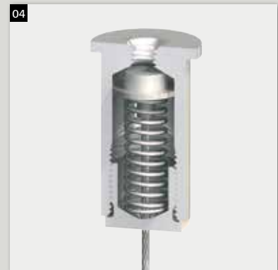
04 Spring tensioner M13x1 nickel plated, combination of ceiling attachment M13x1, washer, spring and screw cap M13x1
