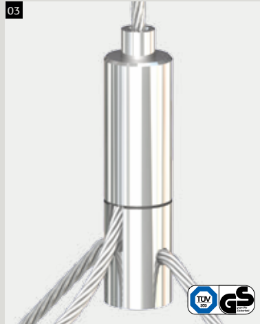
03 Y-Holder type 25 ZW M6i cross hole 3 mm with set screw DIN 915 M6x8
